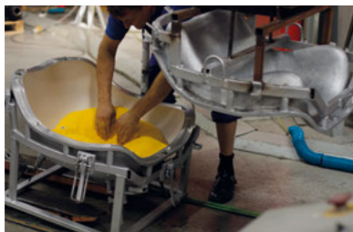
MATRIX FILLED WITH PE POWDER
